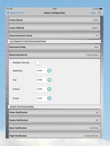
The automatic reporting of the Falcon can also be configured using Single Interval reports, on a range of 10s to 30 min between reports.
