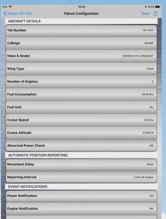
To change the permission for values to be altered, the Falcon will need to be reconfigured via satellite using Air Operations Management with the option "Allow Configuration by Aircrew" enabled.
