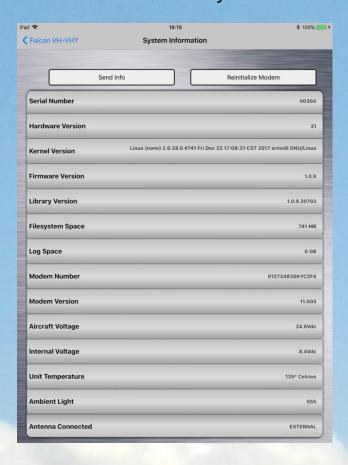
Additionally, the Aircraft Voltage (external power supply) and Internal Voltage values as well as the Unit Temperature can be used to troubleshoot any issues with the performance of the equipment.
